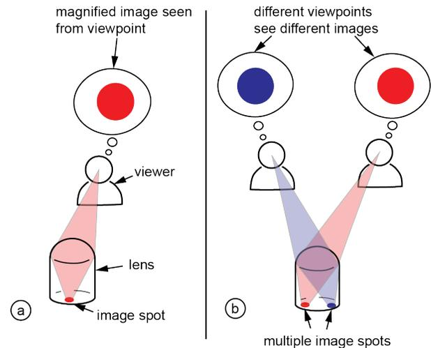
**Figure 2: (a) Magnifying effect of a lens: from each viewpoint, the user sees only a small fraction of the underlying color pattern, i.e. one image spot. (b) From different viewpoints, users see different image spots under the lens, thus from each viewpoint the lens shows a different color.**
