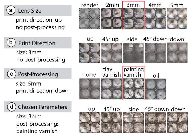
**Figure 5: Fabricated lenses compared with rendered lenses. (a) Larger lenses have better fabrication accuracy, (b) lens quality varies among different printing directions, (c) clay varnish and painting varnish both improve the lens quality, (d) lens quality of our chosen parameters (3mm lenses with painting varnish).**
