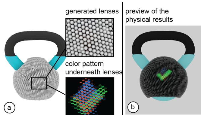
Figure 4: Previewing the resulting object: (a) Generating the lens geometry and underlying color pattern. (b) Simulating the optical result using ray tracing to provide an accurate preview of the object before fabrication.
