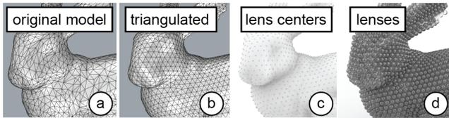
**Figure 10: Placing the lenses: (a) original 3D model, (b) triangular mesh with equilateral triangles, (c) each triangle corner (vertex) is a location for a lens center, (d) lenses placed.**
