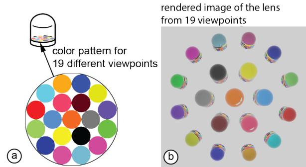
**Figure 9: (a) Our lens geometry allows packing 19 image spots onto the backplane of a lens and thus can support 19 viewpoints with different images; (b) ray traced results of the lens showing 19 different colors from different viewpoints.**
