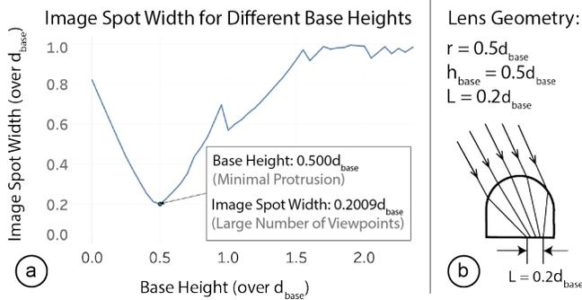
**Figure 8: (a) Finding the base height that minimizes the image spot for  $r = 0.5d_{base}$ ; (b) the resulting lens geometry is  $d_{base} : r : h_{base} = 2 : 1 : 1$ , which results in  $L = 0.2d_{base}$ .**
