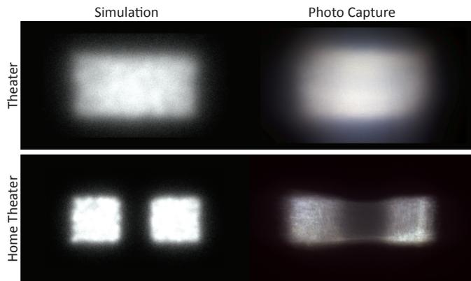
Fig. 17. A directional screen reflection towards the audience. Simulations (left) are compared with fabricated prototypes (right).
