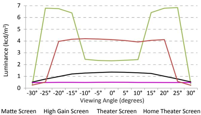
**Fig. 18.** Luminance measurements of home cinema directional screen (green), theater directional screen (red), cinema silver screen (black), and matte screen (purple) across 60 degrees of viewing angle.
