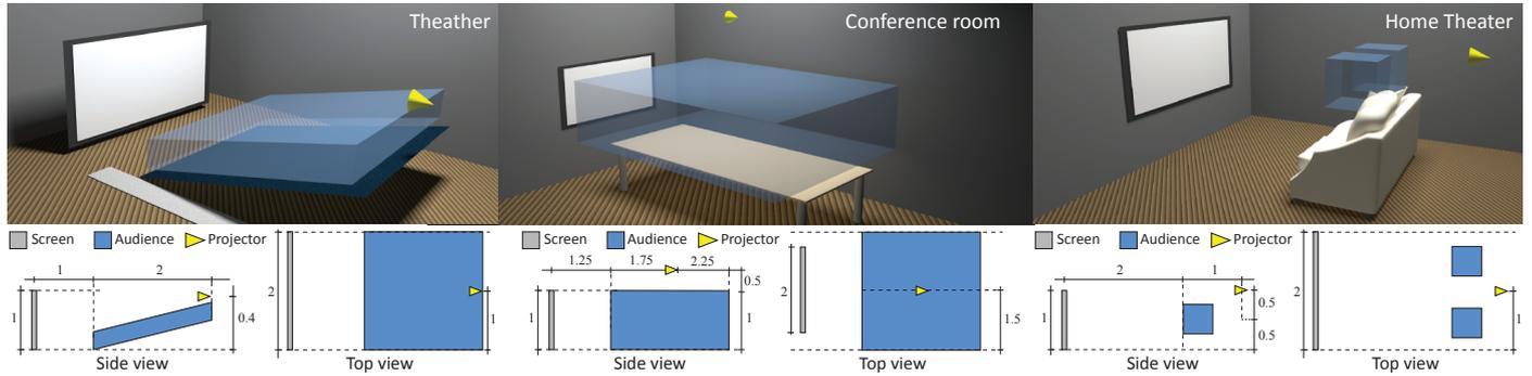
**Fig. 6.** We consider three installations in this paper. The first and the second setup depict one audience, in a theater and in a conference room. The third installation conceives a home theater with two separate audience spaces, for each viewer. Note that the units are left undefined as the design is general and can be scaled to different sizes. This also does not affect our screen computation.
