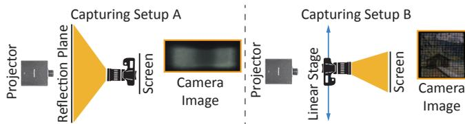
Fig. 16. Prototype capture setup. A camera captures the audience coverage of the examined directional screen (A). A second camera on a linear stage captures the reflection from the directional screen (B).
