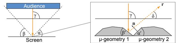
**Fig. 7.** Self-shadowing setup. At each location of the screen the light needs to be reflected to the audience parametrized by opening angles  $\alpha$  and  $\beta$ . A light ray coming from direction  $\gamma$  is reflected from the microgeometry into direction  $\delta$ . Self-shadowing occurs when the reflected angle  $\delta$  is smaller than the angle of neighbouring microgeometry  $\alpha'$ .
