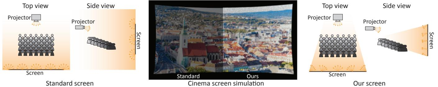
**Fig. 1. Current screens reflect a lot of light into regions where the audience is not expected (left). Reflecting the light toward the ceiling, floor or walls is unnecessary and causes energy loss. Our design enables fine control over the reflectance properties of the screen surface (right), which provides better energy efficiency, brightness, and contrast.**
