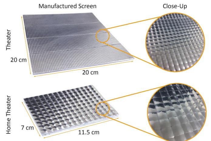
Fig. 15. Photos of manufactured prototypes of a uniform and a split directional screen.
