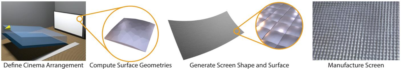
**Fig. 2. Display generation overview:** We start with the definition of the screen, the projector, and the audience. Based on this knowledge we uniformly sample the screen and for each position generate a microgeometry. These geometries are tiled and their heights adjusted to form the final screen surface. The screen surface is manufactured from aluminum on a CNC milling machine.
