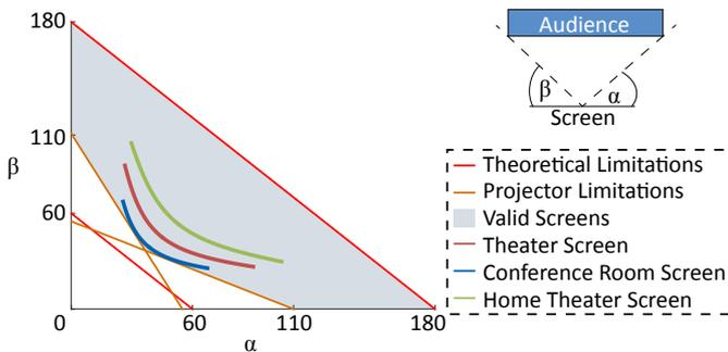
**Fig. 8.** Screen design space plot. Red straight lines mark theoretical limits of directional screens. Orange lines show the gamut of our particular screen-projector setup. Colored curves show our prototype screens. A directional screen reflects light from each point towards the entire audience. At a particular location we can parametrize this reflection by the opening angles  $\alpha$  and  $\beta$ .
