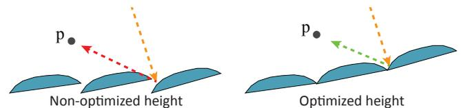
Fig. 5. When the screen surface has discontinuities, shadowing or masking can occur. In this case, a light ray coming from a projector (yellow) should be reflected towards position  $p$ . A discontinuous screen surface may shadow the reflected ray (left). This does not happen when the surface is continuous (right).
