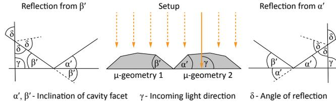
Fig. A.20. Self-shadowing parametrized with facet angle.
