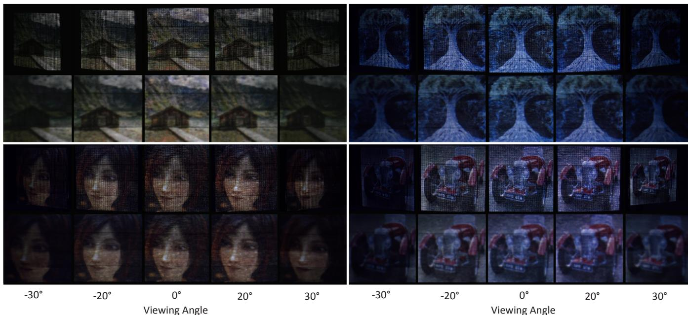
Fig. 14. Manufactured prototype reflecting four images, viewed from various directions, captured by camera setup B. According to the display specification, the reflection should be visible between 0 and 20 degrees (three middle columns). Outside this range (the first and the last column), the image should be dark. The top row of each pair shows raw captures, and the bottom row shows images after applying Gaussian filtering simulating the point spread function of the human eye.
